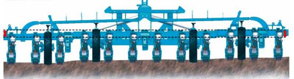
The Compact or Double bar folding frames have independant wings with wheel units. This feature enables a perfect following of the ground contours. In headlands or to finish off a parcel, it is also possible to lift one or other of the wings (or the 2), automatically stopping the seed metering.
