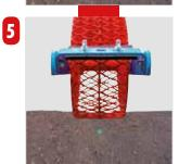
5) The rear wheel closes the furrow around the seed for optimal seed germination.
