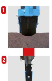
1) The clod remover clears the future planting line of clods or stones whilst the gauge wheel presses the soil and controls the depth.
