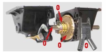
The principle of the Microsem metering resides in the auger system. The microgranules contained in the hopper are taken up by 2 augers (1). The agitators (2) enable a regular feed of these augers. A finger wheel (3) then spread the product uniformly in the chutes (4).
