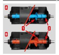
The metering by auger (1), associated with agitators (2), ensure a regular dosing of the fertilizer.
