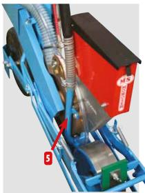
The insecticide Microsem tube (5) is placed just behind the shoe so as to distribute the product in the planting line.
