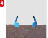
4) The scrapers\* (retractable if necessary) scrape fine soil over the seeds.
