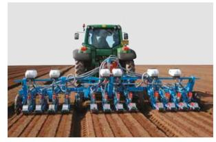
$MS\ C\ Planter$  - Double bar folding frame - 3 x 4 rows with Microsem
