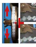
The selection adjustment is made using a single lever which is easily accessible on the top of the metering boxes. The quality and the precision of the MS metering boxes enables an identical adjustment on all of the units.
