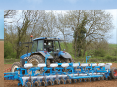
Mechanical planter for pelleted sugarbeet MECA V4
