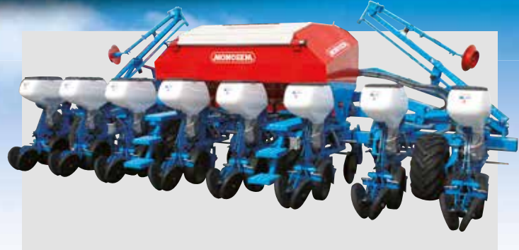
8-row TFC floating frame (75 cm inter row spacing)
