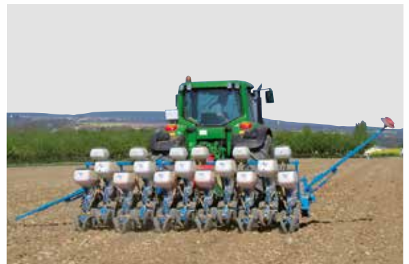
11-row rigid Monoblock planter (37,5 cm inter row spacings or 6 rows at 75 cm inter row spacing)
