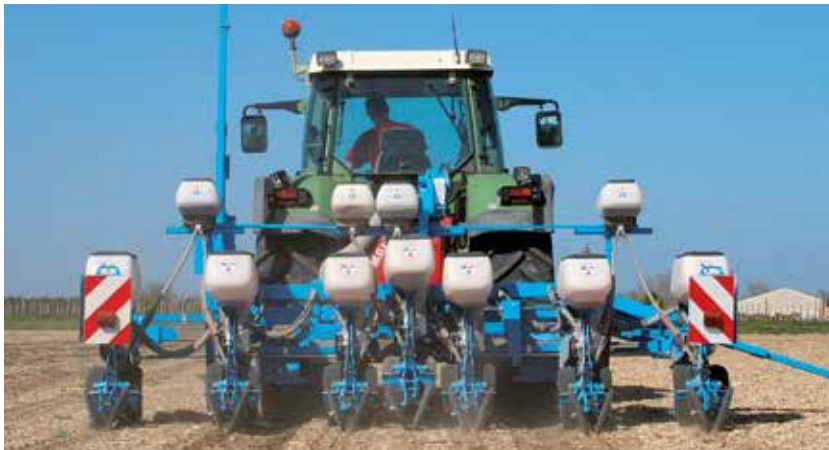
The mixed 6/7 row Extend version offers spacings of 75 and 80 cm in 6 rows and of 55 and 60 cm in 7 rows. It is thus possible to change very quickly with no disassembly, from 6 rows maize to 7 rows sunflower/rapeseed.
