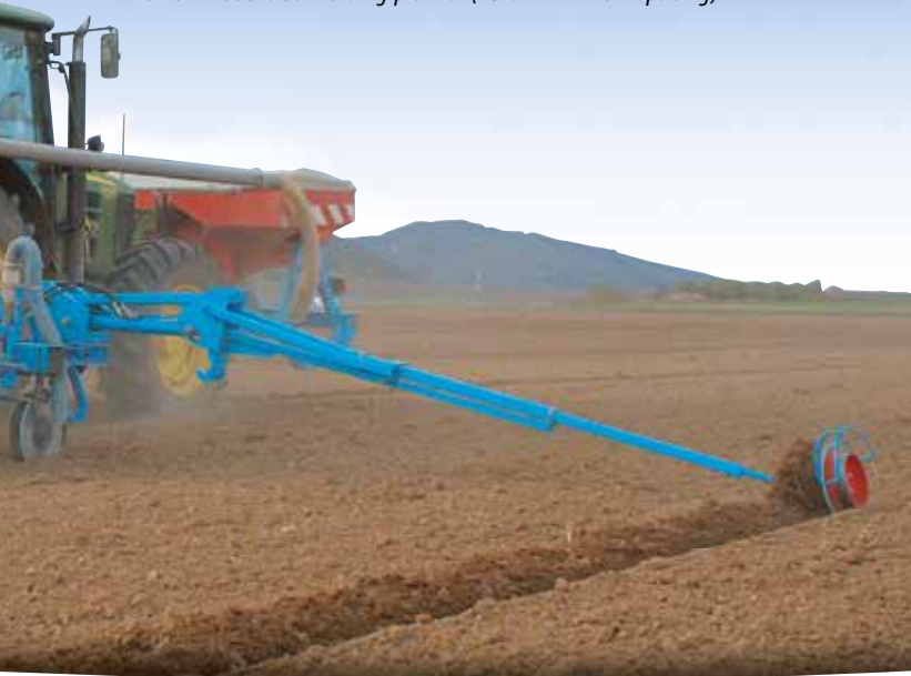
8-row Double bar folding planter (75 cm inter row spacing)
