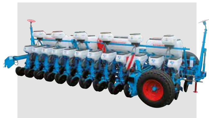
12-row rigid Double bar planter (45 cm inter row spacing) with lengthwise transport carriage
