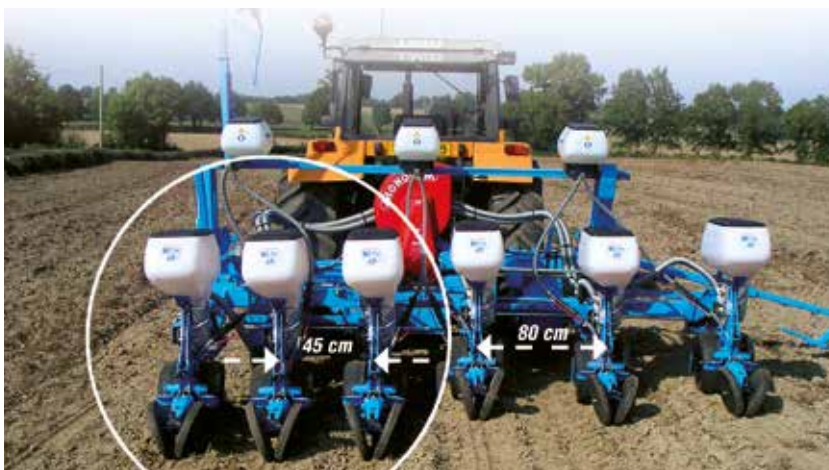
The 6-row Extend planter enables spacings of 45, 50, 55, 60, 65, 70, 75 and 80 cm.
