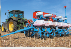
Special pneumatic « low-till » planter Monoshox NX M with discs
