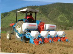
Multi-purpose pneumatic planter with NC shoes
