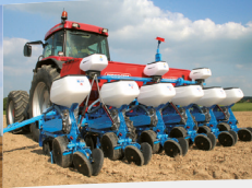
Multi-purpose pneumatic NG Plus 4 planter with discs
