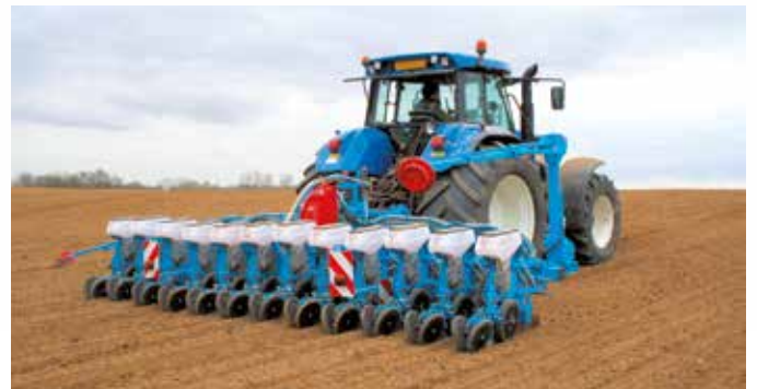
12-row Double bar folding planter (45 cm inter row spacing)
