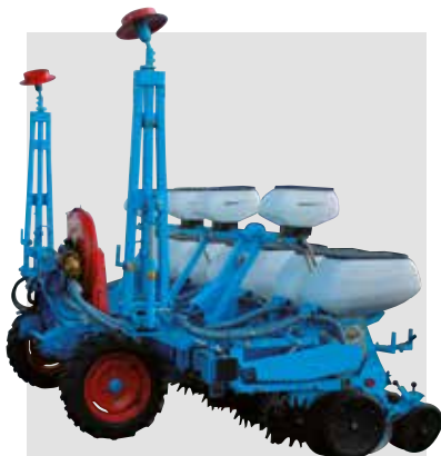
The Monoblock frame long off-set with front wheel unit enables reduced inter row spacings of 37,5 cm.
